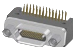
CONDENSED BOARD RIGHT ANGLE TYPE (CBR) 0.050" PITCH
