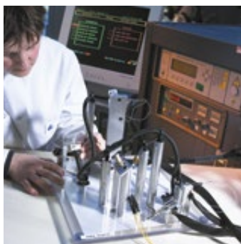
▲ AUTOMATIC CONTINUITY & INSULATION RESISTANCE TEST
